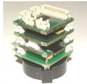
Fig. 1. 25mm prototype module with coin battery
